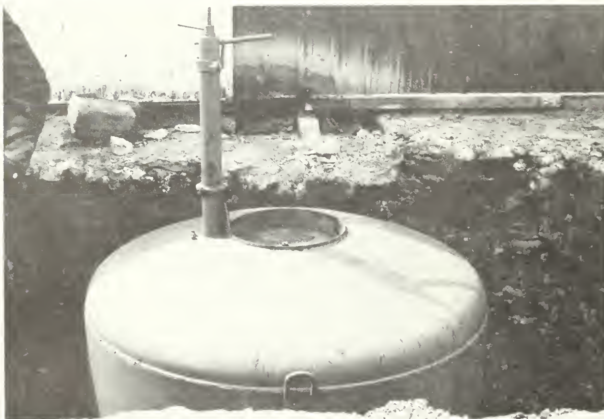
Figure 3.5.19 Pneumatic pressure vessel for transferring manure to storage tank (courtesy Patz Company)
